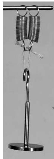
What is the total strain energy stored with two springs arranged in this way?
