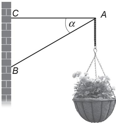
Given that the mass of the hanging basket is 3.6 kg, calculate the thrust in the rod  $AB$  and the tension in the rod  $AC$ . [5]
