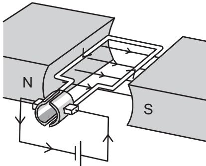
Use the diagram to explain how rotation is caused in the motor.
