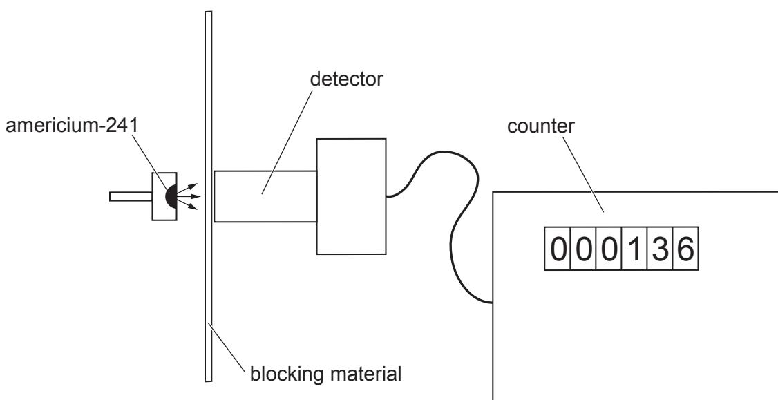
They recorded the number of counts detected in one minute with different blocking materials.
