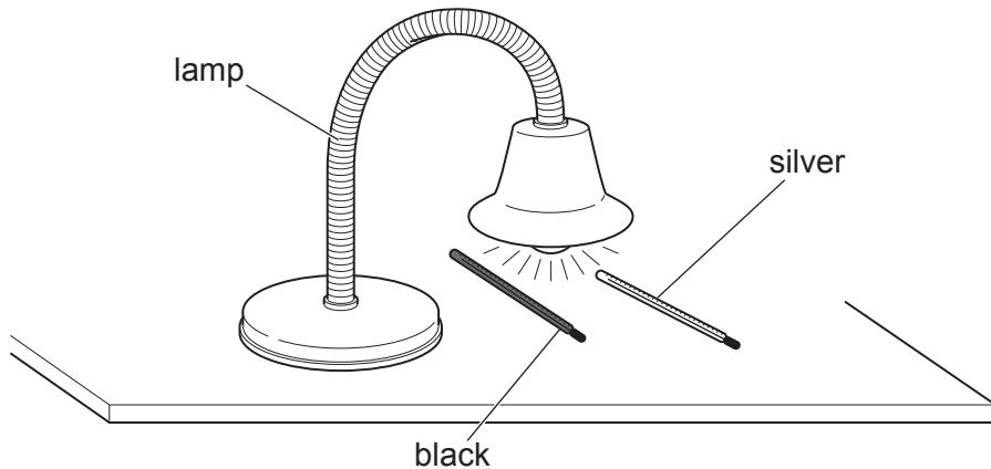
He records how the temperature of each thermometer changes over four minutes.
