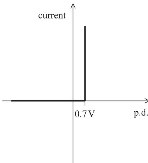
(a) Describe how the current through this diode varies for positive p.d.s and negative p.d.s. (2)
