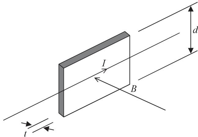
Electrons collect at the top edge of the slice and the bottom edge becomes positively charged. As a result a potential difference known as a Hall voltage  $V_{\text{HALL}}$  develops.
