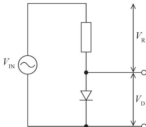
The p.d. across the resistor is  $V_R$  and the p.d. across the diode is  $V_D$ .  $V_D$  is the output.
