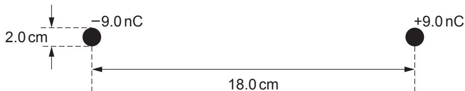
(a) (i) Show that the potential at the surface of the negative sphere is approximately  $-7500 \text{ V}$ . [3]
