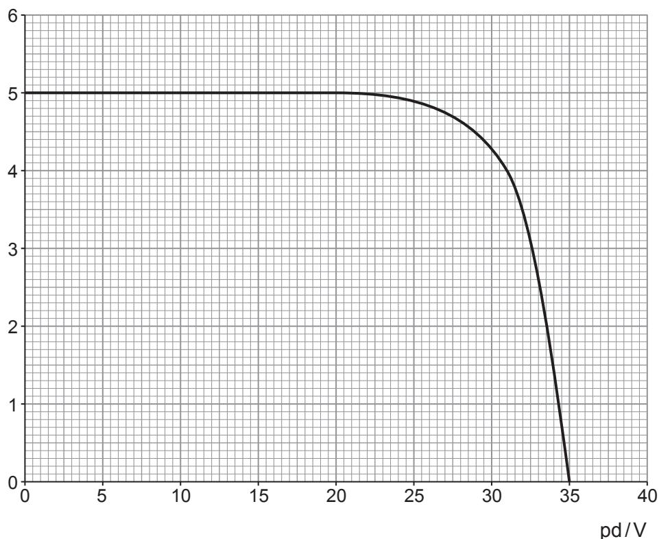
The solar panel has a surface area of  $1.2 \text{ m}^2$ . Determine the efficiency of the solar panel when it is operating at its maximum power output. [4]
