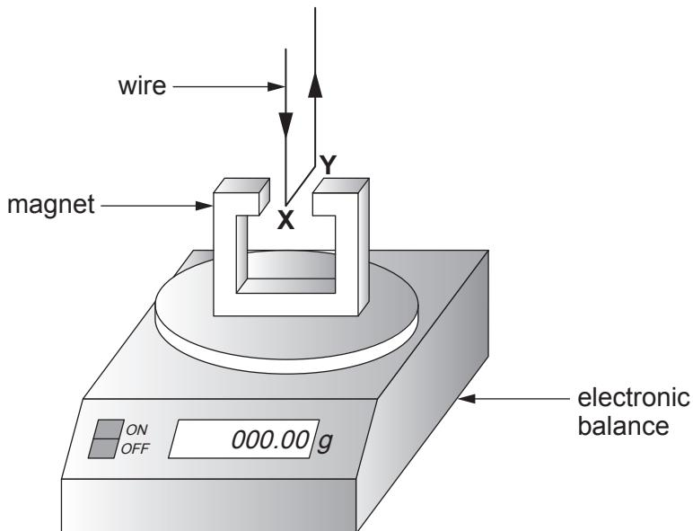
The part **XY** of the wire which is in the magnetic field, has been placed carefully so that the current is from front to back at  $90^\circ$  to the direction of the magnetic field. When there is no current the balance is reset to display 000.00 g. When there is a current in the direction shown, the magnetic force results in a positive reading on the display of the balance. However, this signifies an upward force on the wire.
