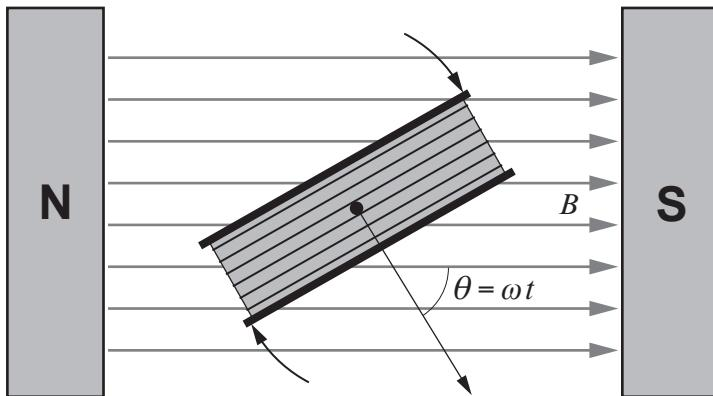
The coil rotates 50 times per second in a field of flux density 0.215 T. The coil has 2650 turns and cross-sectional area  $2.35 \times 10^{-3} \text{ m}^2$ . (Note that  $\theta = 0$  when  $t = 0$ )
