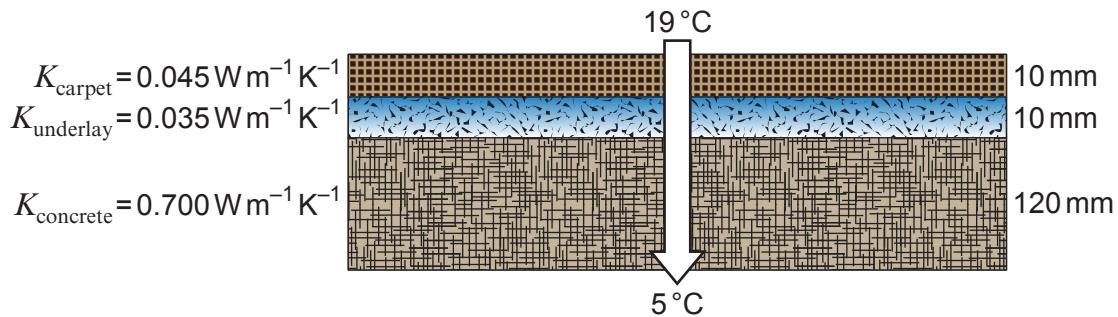
It is stated by the carpet fitting company that the rate of heat flow through the floor will reduce to a quarter of the value calculated in part (d)(i). Evaluate if this claim is correct. [3]
