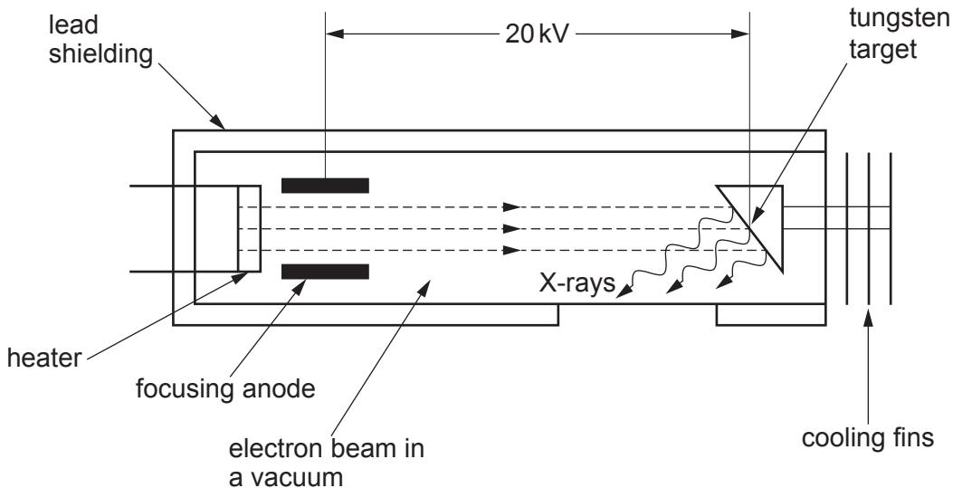
(i) State the main function of the heater **and** explain why there must be a vacuum between the heater and the tungsten target. [2]
